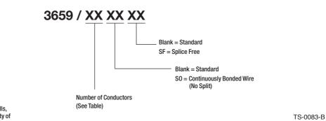
Note: Available in standard lengths of 100 ft or 300 ft rolls, please specify when ordering. Contact 3M for availability of additional conductor counts and/or custom roll lengths.
