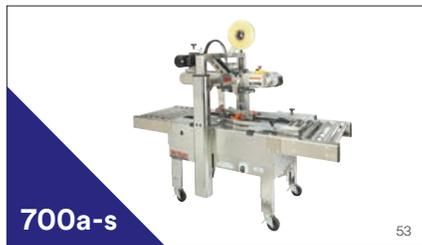
**3M-Matic™ Adjustable Case Sealer 700a-s** has advanced features to seal uniform cases at up to 30 per minute. Dual masts with dual lead screws for stability and uniform height adjustments. Adjustable top and bottom belt drive system for reliable conveyance of heavier or tall/light boxes. Compression rollers position each box for precise tape sealing. Stainless construction for corrosive environments.
