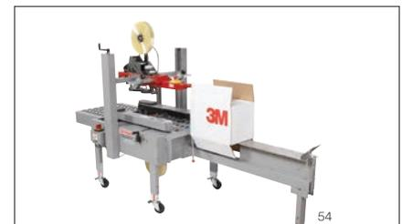
**3M-Matic™ T-table Attachment** is a 6" x 44" t-table attachment for use with 3M-Matic™ Case Sealers a80 and a80-3.
