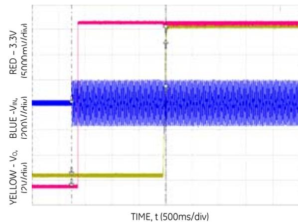
Figure 5. Typical Start-up ( $V_{IN} = 230V_{ac}$ ).
