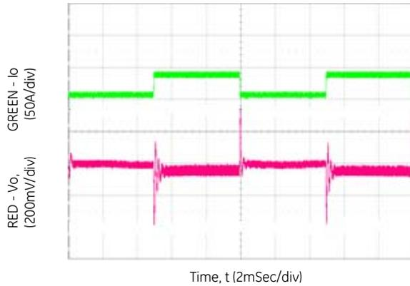
Figure 9. 10%-60%-10% Load Transient, Slew Rate = 1A/uS, V<sub>IN</sub> = 230V<sub>ac</sub>, V<sub>o</sub> = 12V<sub>dc</sub>
