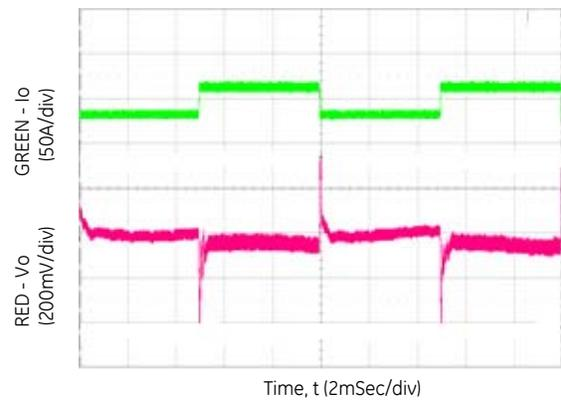
Figure 10. 50%-100%-50% Load Transient, Slew Rate = 1A/uS, V<sub>IN</sub> = 230V<sub>ac</sub>, V<sub>o</sub> = 12V<sub>dc</sub>
