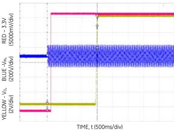
Figure 6. Typical Start-up ( $V_{IN} = 150V_{ac}$ ).
