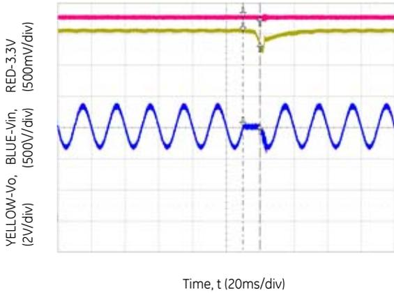
Figure 7. Ride Through at full load, V<sub>IN</sub> = 230V<sub>ac</sub>, V<sub>o</sub> = 12V<sub>dc</sub>.
