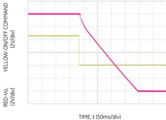
Figure 12. 12V<sub>dc</sub> Turn-off delay upon inception of ON/OFF command, Vin = 230V
