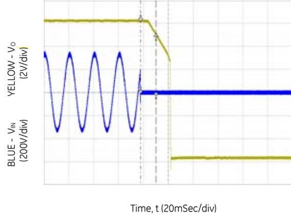
Figure 8. Hold up at 50A load, V<sub>IN</sub> = 230V<sub>ac</sub>, V<sub>o</sub> = 12V<sub>dc</sub>
