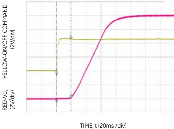
Figure 11. 12V<sub>dc</sub> Turn-on delay upon inception of ON/OFF command, Vin = 230V
