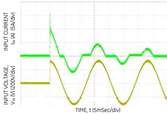
Figure 2. Inrush Current ( $V_{IN} = 230V_{ac}$ , 100% load)
