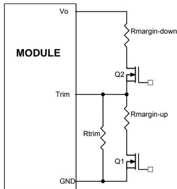
Figure 46. Circuit Configuration for margining Output voltage.
