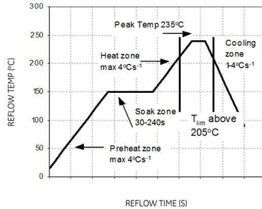
Figure 15: Reflow Profile for Tin/Lead (Sn/Pb) process.
