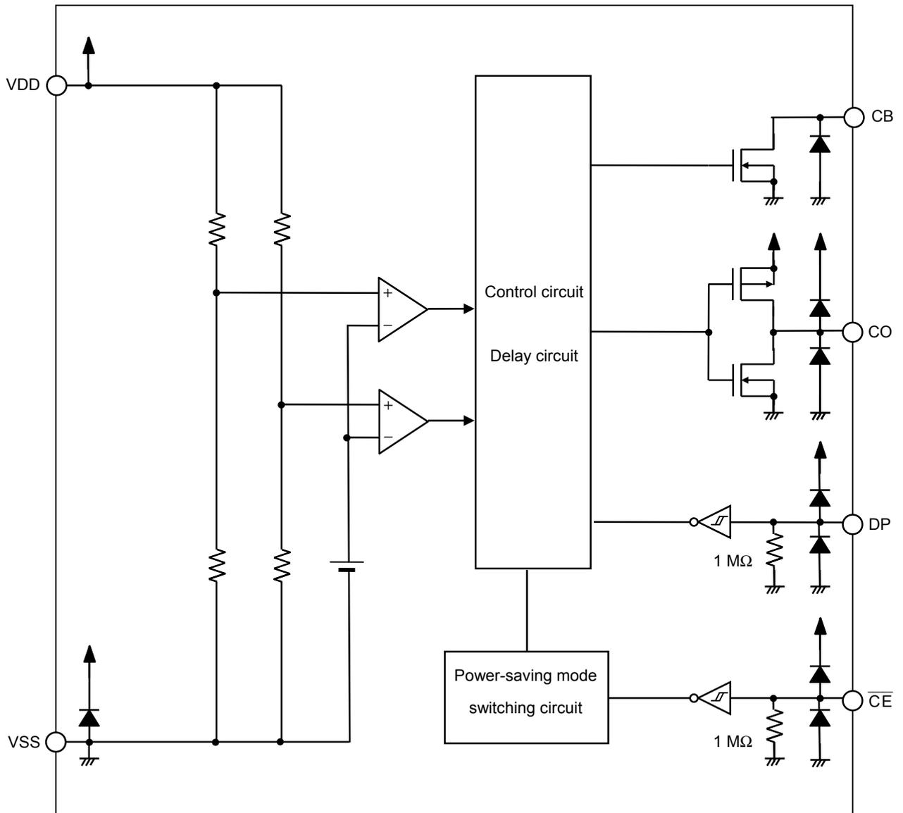
\*1. All diodes shown in the figure are parasitic diodes.
