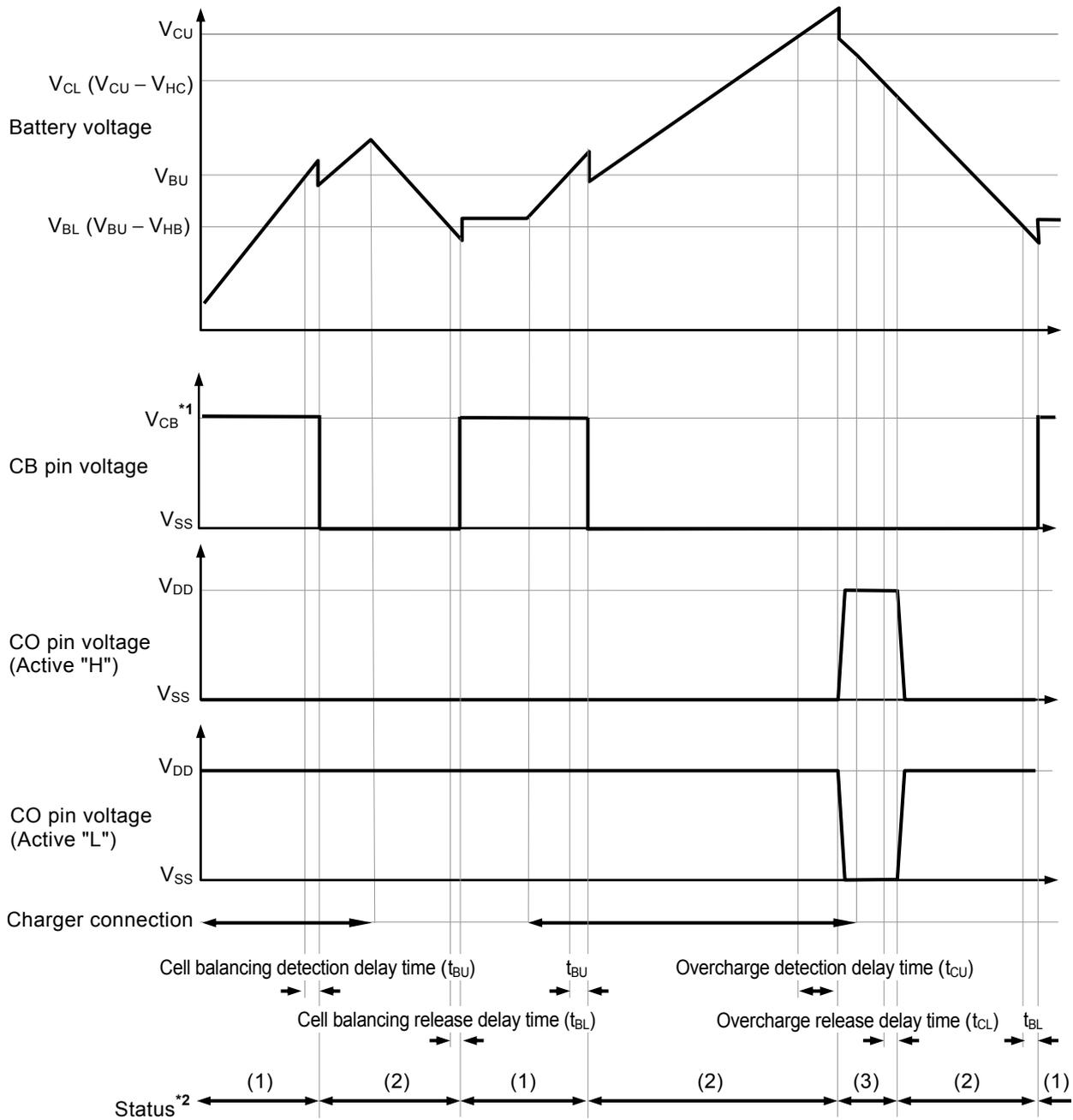
\*1. The CB pin is pulled up by the external resistor.
