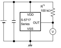
\*1. Resistor (R) is unnecessary for the CMOS output product.
