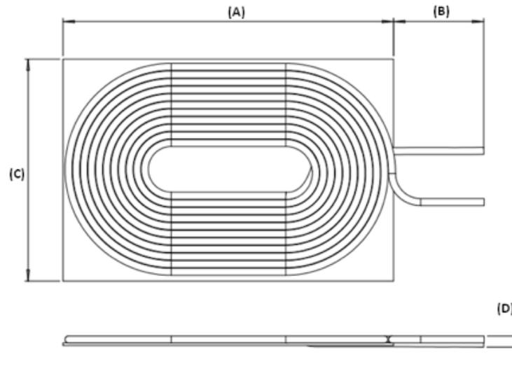
\* Coiled wire has been pressed together to reduce thickness where wire overlaps
