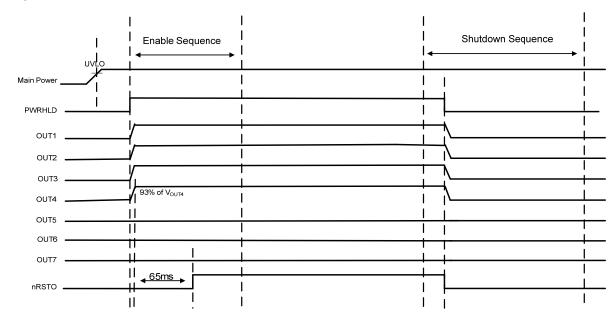
Remark: 1, Reset signal is triggered by OUT4 output, no PWREN function for standby.
