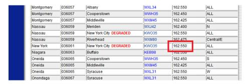
The frequency is 162.550 MHz, type that into the SDR# frequency window
