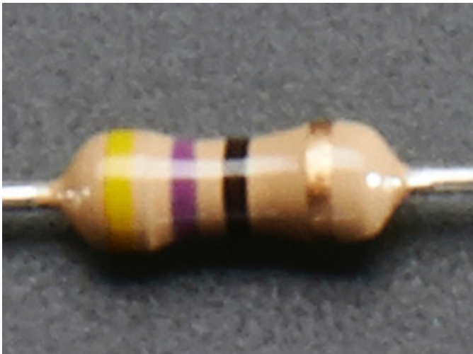
10x 47ohm 5% 1/4W Resistor
