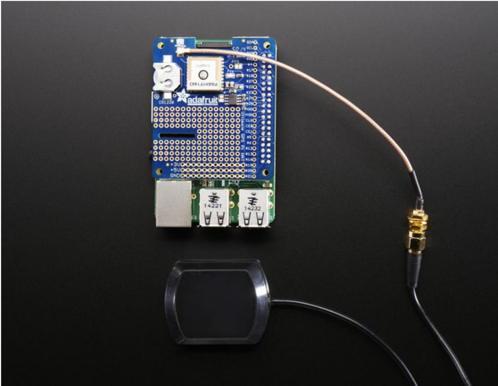
All Ultimate GPS modules have a built in patch antenna - this antenna provides -165 dBm sensitivity and is perfect for many projects. However, if you want to place your project in a box, it might not be possible to have the antenna pointing up, or it might be in a metal shield, or you may need more sensitivity. In these cases, [you may want to use an external active antenna. \(http://adafru.it/960\)](http://adafru.it/960)
