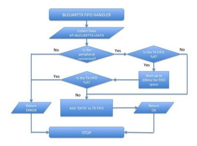
Note: The TX FIFO full check will happen for each GATT transaction (of up to 20 bytes of data each), so large data transfers may have multiple 200ms wait states.
