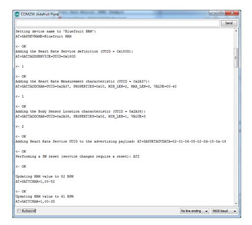
If you open up an application on your mobile device or laptop that support the standard Heart Rate Monitor Service (https://adafru.it/f4l), you should be able to see the heart rate being updated in sync with the changes seen in the Serial Monitor:
