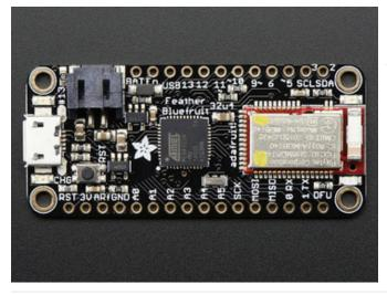
Bluefruit Micro or Feather 32u4 Bluefruit If you have a Bluefruit Micro or Feather 32u4 Bluefruit LE then you have an **ATmega32u4** chip with **Hardware SPI**, CS = **8**, IRQ = **7**, RST = **4**
