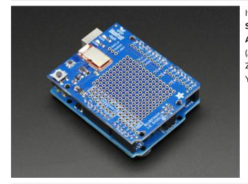
If you are using the Bluefruit LE Shield then you have an SPI-connected NRF51822 module. You can use this with Atmega328 (Arduino UNO or compatible), ATmega32u4 (Arduino Leonardo, compatible) or ATSAMD21 (Arduino Zero, compatible) and possibly others. Your pinouts are Hardware SPI, CS = 8, IRQ = 7, RST = 4
