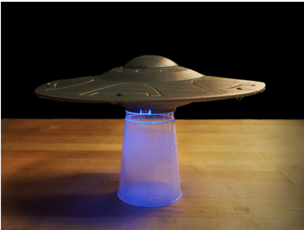
UFO Flying Saucer ( https://adafru.it/BeJ ) by John Park ( https://adafru.it/Ch7 ) uses the accelerometer tilt to control lights and sounds on a fun flying saucer.
