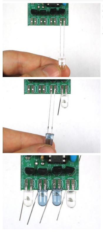
Next is the IR LEDs. Start with **LED1**, a clear IR led. Like the small indicator LED, it has polarity. Make sure the longer, positive lead is on the right, as shown.
