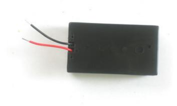
Strip the ends of the wire off so that there's a short section without insulation.
