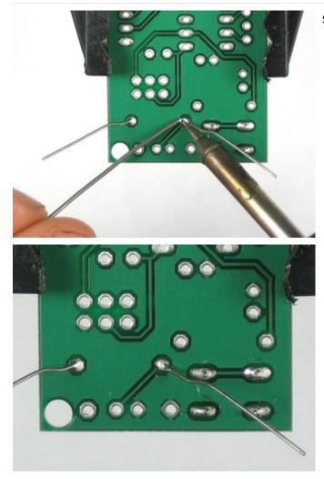
Solder each leg of the resistor.
