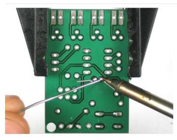
Solder and clip the ceramic capacitor part.
