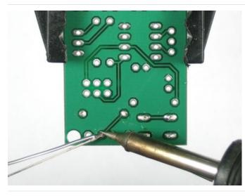
Turn the PCB over and solder both leads of the LED.
