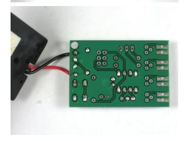
Insert the wires into the PCB so that the red wire goes to the + hole and the black wire goes to the - hole.
