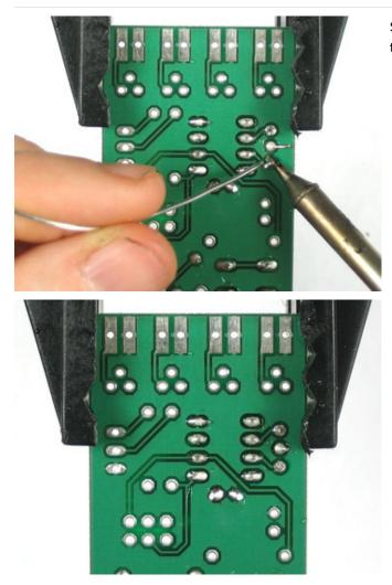
Solder the rest of the points then clip short the legs of the oscillator.
