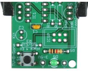
The next part is the ceramic capacitor **C1**. Ceramic capacitors are symmetric so it can go in either way.
