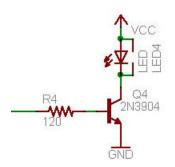
The IR LEDs have more than 100mA going through them. This is way more than a microcontroller pin can supply (usually 20 to 40 mA max!) so we use a 'driving' transistor. These NPN transistors amplify the power of a microcontroller pin and are designed to turn off currents of over 100mA. When the base pin is pulled high (though the base resistor) the transistor turns on and the LED turns on too. When the base pin is pulled to ground, the transistor turns off and no current passes through the LED.
