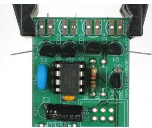
Next are the four NPN (2N2222) transistors **Q1 Q2 Q3** and **Q4**. These are the devices that turn on and off the high power IR LEDs. The microcontroller doesn't have the capability to provide a lot of power directly to the LEDs so these transistors assist it.
