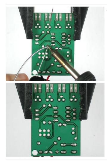
Solder and clip the resistor.
