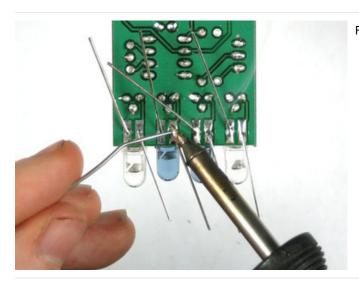
Flip over the PCB and solder it to the bottom.
