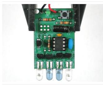
If you're in the EU, UK, Australia, place the remaining 10K resistor into **R3.** This will tell the micrcontroller to use the EU database.
