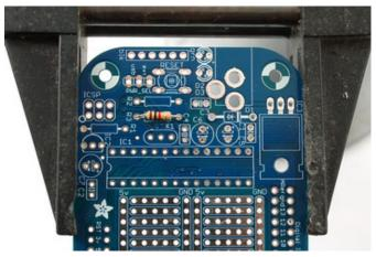
The first component we will be placing is called **R3** and it's right in the middle of the PCB. **R3** is a 1000 ohm (1Kohm) resistor - with Brown, Black, Red, Gold stripes. Be careful you don't confuse it with the 10K resistor which has an orange stripe. If you're not sure, use a multimeter to check!
