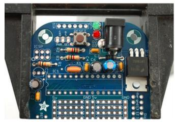
lets the Menta chip run at a brisk 16 million clocks per second. This oscillator comes in a orange shape with three pins. Luckily, it's symmetric so just place it any way you like.
