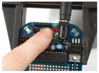
Now we can do a second test, to check the chip and crystal are working right. Plug in the board again to the DC power and press the reset button, you should see the red LED flashing a few times. Every time you press the button it should flash again.
