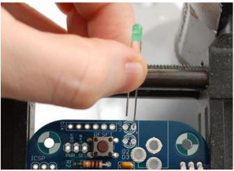
Now we will solder in the indicator LEDs. These LEDs are the Menta's way of telling you what's going on. LEDs are Light Emitting Diodes - which means that like the 1N4001 they have a polarity and won't work if placed backwards. Like capacitors, the also have a longer wire that indicates the **positive** lead. Place this wire in the hole marked with a +.
