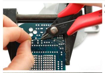
Using your diagonal cutters, cut off the long leads just above the solder joint.
