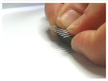
Now we can place the ATmega328 chip - the brains of the Menta. Chips come with the legs in an A shape, but we want it in more of an H shape. Pick the chip out of the antistatic foam and holding it by the ends, bend the leads against the table to flatten them parallel.
