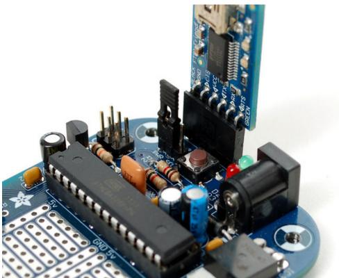
Connect the FTDI adapter to your computer and start the IDE. Select the **COM** or /dev/tty port that is created when you plugged in the FTDI adapter.
