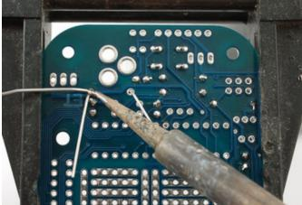
Now we will place our first non-symmetric component, a diode! The diode only conducts current in one direction. We use this diode for protecting the Menta - since it can only work in one direction it makes sure we don't connect negative voltages into the DC plug that could damage or destroy the electronics. This particular diode is a **1N4001** model, which is extremely common power diode that can handle over an Amp of current.
