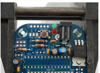
Now we can place the big power jack. This is how we can plug in a battery or power adapter.
