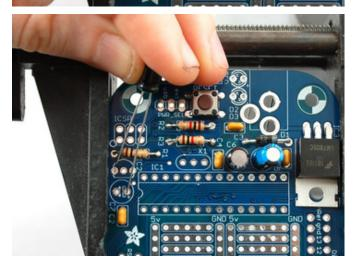
Next we will place the polarized electrolytic capacitors. These are the beefy versions of the ceramic capacitors we already placed. Ceramics are good for high frequency noise, and the electrolytics are good for low frequency noise, that's why we team them up together to cover all frequencies.
