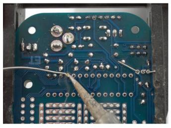
Solder in all 28 pins of the socket and the 3.3V regulator.
