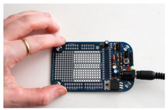
Now we can do a test, find a DC power adapter, 7VDC or higher, with a 2.1mm jack and center-polarity (these are nearly standard) and plug it in. With the jumper in place, you should see the Green LED light up. If not, something is wrong - either the LED is in backwards or your power supply isn't working. Go back and check your work until you can figure out what happened.
