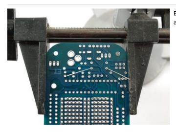
Bend out the long metal leads so the resistor sits flat agains the board, and flip the PCB over.
