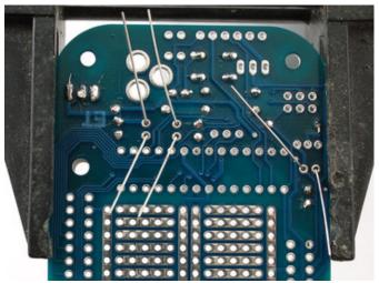
After you've triple-checked the polarity of the capacitors, flip over the PCB and solder them in.
