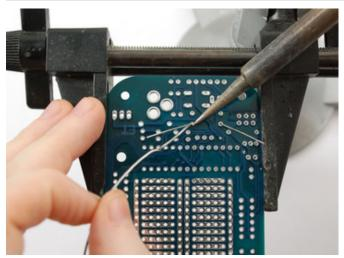
Now we will solder in the first part. Heat up your soldering iron (about 700 degrees F is common but you may need to adjust it higher for lead-free).
