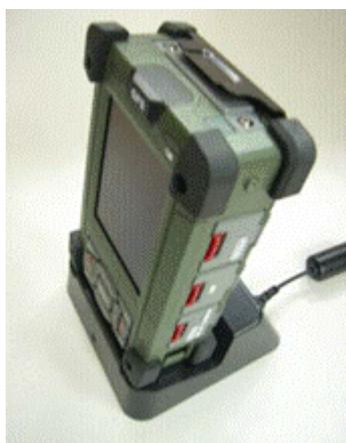
3. Plug the power cable connector into the AC adapter (B), Plug the AC adapter into an electrical outlet (C).
