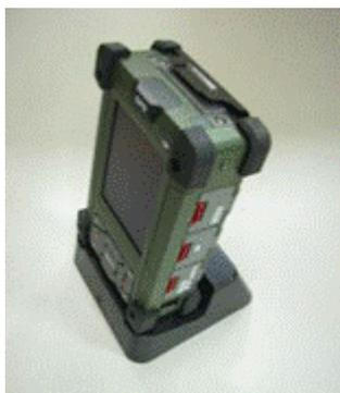
2. Plug the AC adapter cable into the power connector on the cradle (A).
