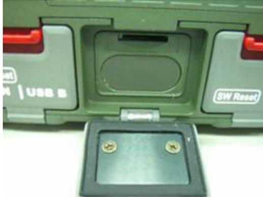
2. Insert the Micro SD card with the notched corner as oriented as shown below.
