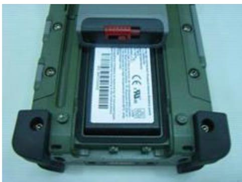
3. Replace the battery compartment cover, and lock the battery latch.
