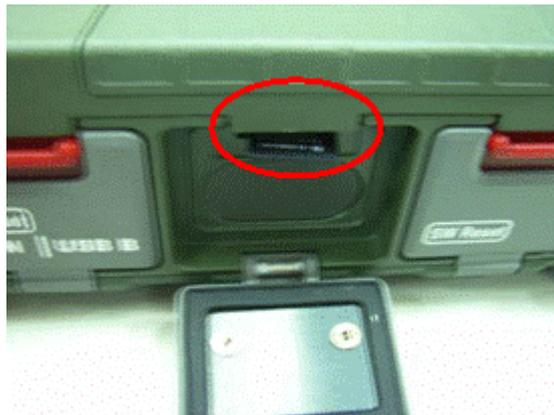
3. Press the card into the slot. The card is secure when it is flush with the slot.
