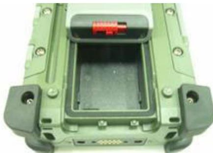
2. Align the battery contacts with the contacts in the compartment and place the battery in the compartment as shown below.
