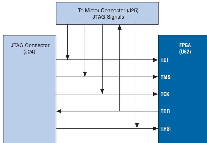
**Figure 2–19. USB Blaster Connected to J24 JTAG Connector**
