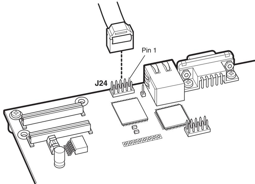
The FPGA's JTAG pins can also be accessed via the Mictor connector (J25). The pins of J24 are connected directly to pins on J25, and care must be taken so that signal contention does not occur between the two connectors.
