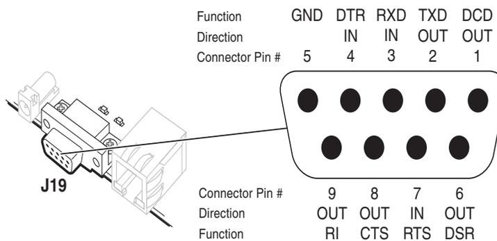
**Table 2–10. Serial Connector Pin Table**
