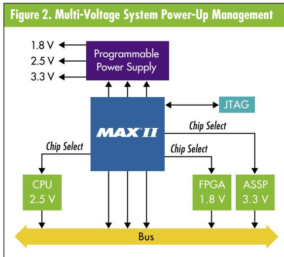
onboard user flash memory can record a log of when each board is plugged into and out of the backplane. The MAX II device family also supports hot socketing, where devices can be plugged into and out of a live system without damage to the core or requirements for special plug layout.
