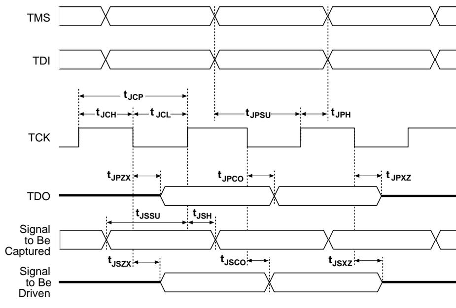
Table 11 shows the JTAG timing parameters and values for MAX 7000A devices.
