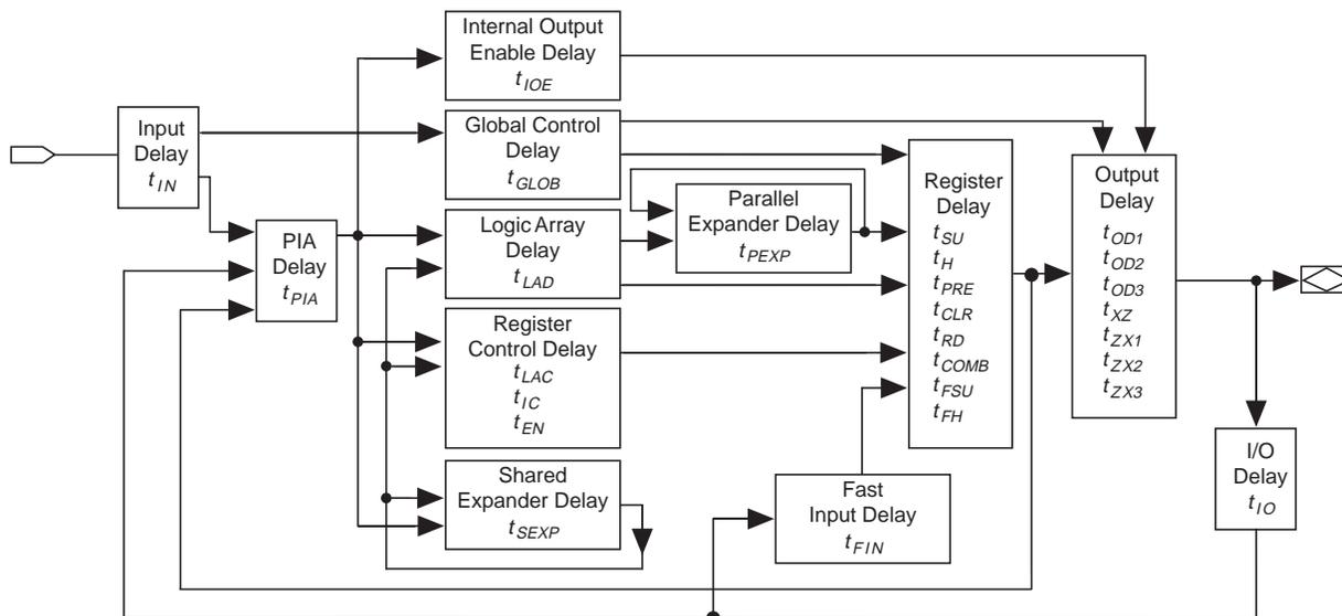
The timing characteristics of any signal path can be derived from the timing model and parameters of a particular device. External timing parameters, which represent pin-to-pin timing delays, can be calculated as the sum of internal parameters. Figure 12 shows the timing relationship between internal and external delay parameters.
