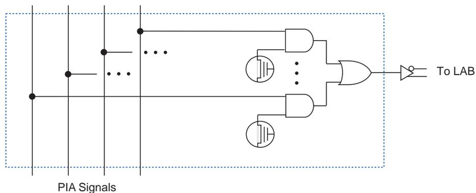
While the routing delays of channel-based routing schemes in masked or FPGAs are cumulative, variable, and path-dependent, the MAX 7000A PIA has a predictable delay. The PIA makes a design's timing performance easy to predict.
