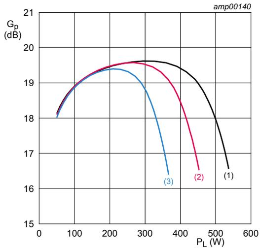
$I_{Dq} = 90 \text{ mA}; f = 915 \text{ MHz.}$
