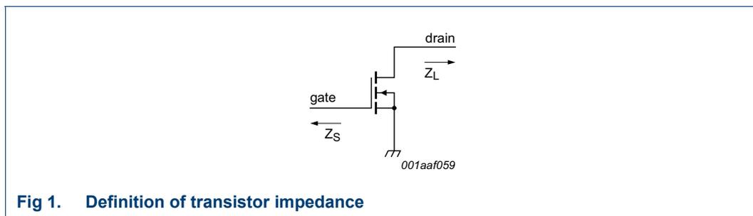
Fig 1. Definition of transistor impedance
