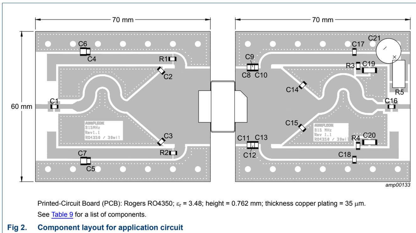
Printed-Circuit Board (PCB): Rogers RO4350;  $\epsilon_r = 3.48$ ; height = 0.762 mm; thickness copper plating = 35  $\mu\text{m}$ .
