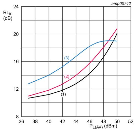
$V_{DS} = 28\text{ V}$ ;  $I_{Dq} = 120\text{ mA}$ ;  $V_{GS(amp)peak} = 0.8\text{ V}$ ; 46 % clipping.
