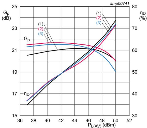
$V_{DS} = 28\text{ V}$ ;  $I_{Dq} = 120\text{ mA}$ ;  $V_{GS(amp)peak} = 0.8\text{ V}$ ; 46 % clipping.
