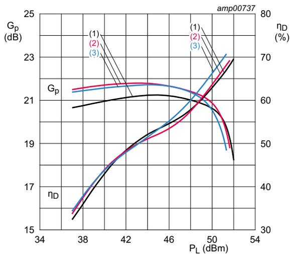
$V_{DS} = 28 \text{ V}$ ;  $I_{Dq} = 120 \text{ mA}$ ;  $V_{GS(amp)peak} = 0.8 \text{ V}$ .
