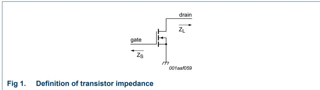
Fig 1. Definition of transistor impedance
