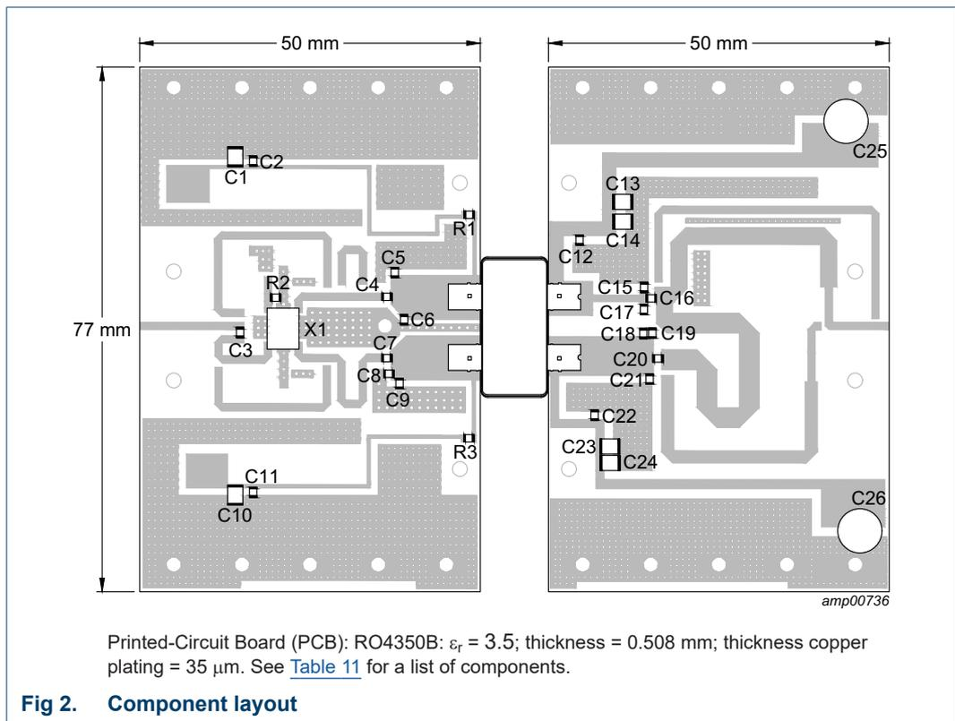
Printed-Circuit Board (PCB): RO4350B:  $\epsilon_r = 3.5$ ; thickness = 0.508 mm; thickness copper plating = 35  $\mu\text{m}$ . See [Table 11](#) for a list of components.
