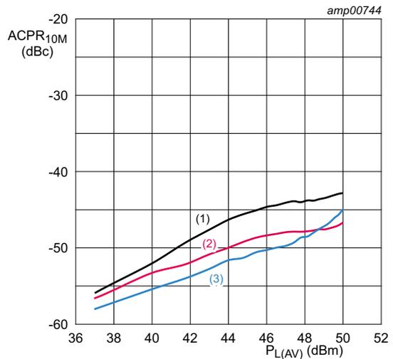
$V_{DS} = 28\text{ V}$ ;  $I_{Dq} = 120\text{ mA}$ ;  $V_{GS(amp)peak} = 0.8\text{ V}$ ; 46 % clipping.
