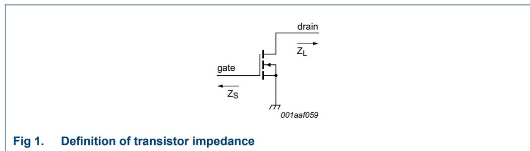
**Fig 1. Definition of transistor impedance**
