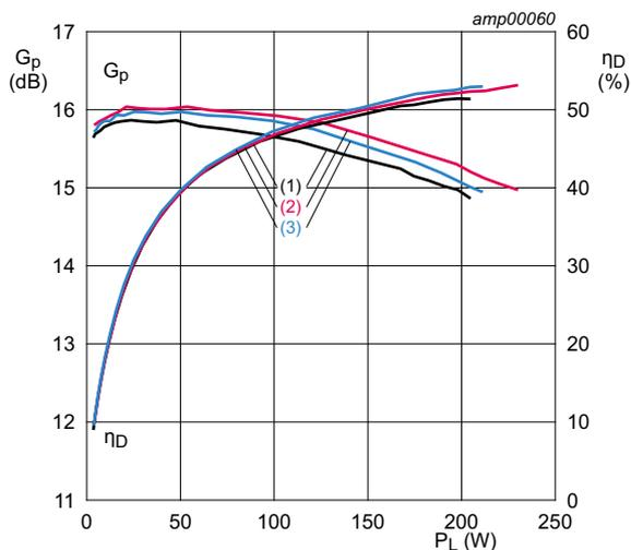
$V_{DS} = 32\text{ V}; I_{Dq} = 850\text{ mA}; V_{GS(amp)peak} = 0.6\text{ V}.$
