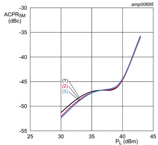
$V_{DS} = 50\text{ V}; I_{Dq} = 115\text{ mA}.$
