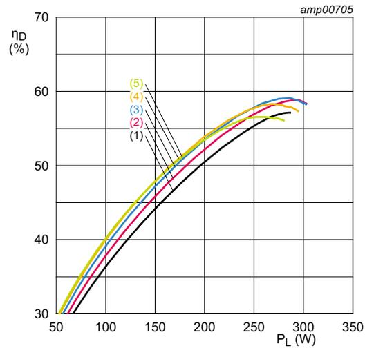
$I_{Dq1} = 25 \text{ mA}; I_{Dq2} = 50 \text{ mA}; V_{DS} = 32 \text{ V}; T_{mb} = 25 \text{ }^\circ\text{C}.$
