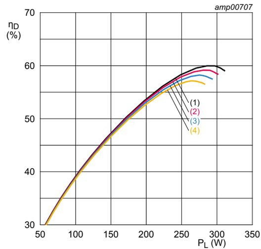
$I_{Dq1} = 25 \text{ mA}; I_{Dq2} = 50 \text{ mA}; V_{DS} = 32 \text{ V}; f = 2450 \text{ MHz}.$
