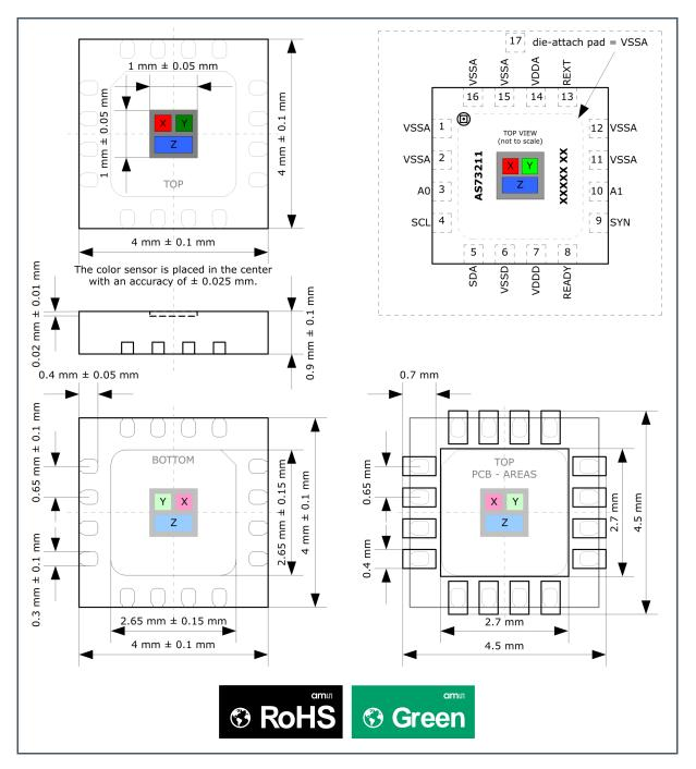
(1) All dimensions are in millimeters. Angles in degrees.
