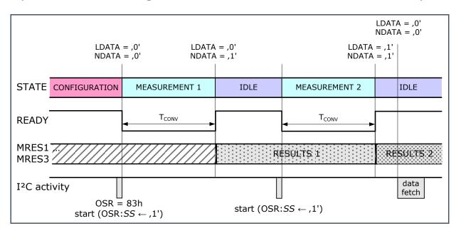
The status bits STATUS:STANDBYSTATE and STATUS:POWERSTATE always show the actual status of the internal control signals for Standby and Power Down. In both cases it can differ from the actual set bits CREG3:SB and OSR:PD, because of the behavior of the control signals while a measurement is in process. The reading of the 16-bit values of the output result registers always starts with the least significant byte.
