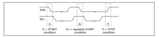
After the protocol started, the data at pin SDA must be stable as long as the high phase of I<sup>2</sup>C clock at pin SCL takes. The change of the communication data at pin SDA is only allowed during the low phase of SCL clock.
