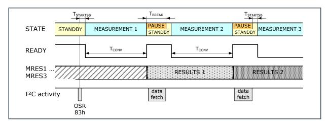
Another example shows, that after the end of a conversion in CMD mode the AS73211 returns to Power Down and/or Standby state depending on the bits OSR:PD and CREG3:SB. In case of both bits are ,0' while in Measurement state the device would return to idle, waiting for the next measurement to start. Figure 24: Principle sequence whereas measurement starts in CMD mode with Power Down and Standby switched on (device is already in Measurement state):
