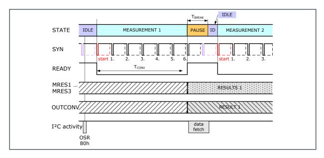
The conversion time (TCONV) is determined by the duration between the edges of start and stop of the signal SYN. If CREG2:EN\_TM is set to ,1', the register OUTCONV contains an equivalent amount of TCONV as counts of the internal clock. With the value of OUTCONV, the measurement results can be calculated more precisely (see chapter "Conversion Time Measurement in SYND Mode").
