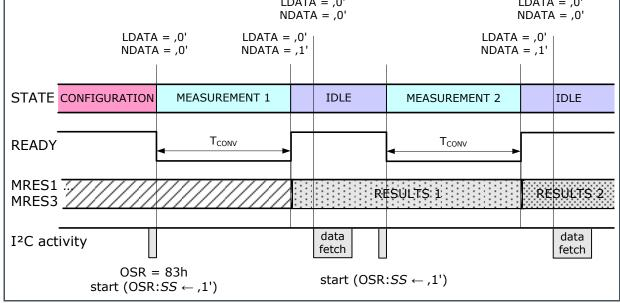
If the buffer registers contain new values (NDATA = ,1') and then a new measurement finishes before an I<sup>2</sup>C reading process occurs, the new measurement results is stored in the buffer registers. The older measurement results are overwritten. The status bit LDATA as shown in Figure 56 indicates this. The LDATA bit is only reset to ,0' by reading the status register, because it allows checking for the loss of information after multiple measurement cycles.
