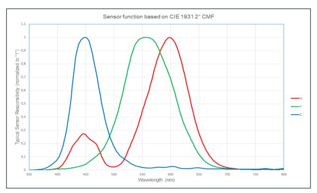
Typical characteristic sensitivity. Spectral tolerance filter curve Δλ(λ) typ. <±1%\*λ determined by the deviation between the filter curve's centroid wavelength and the CIE 1931 2° Standard Observer centroid wavelength.</li>
