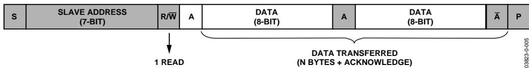
Figure 25. I<sup>2</sup>C—Master Reading Data from Slave
