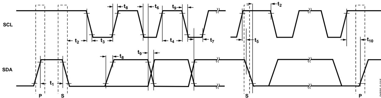
Figure 2. I<sup>2</sup>C Timing Diagram
