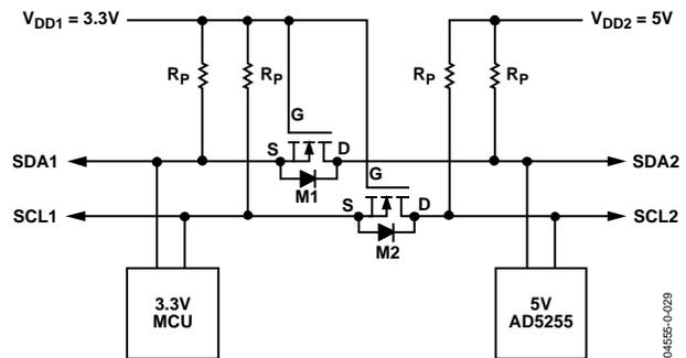
Figure 29. Level Shifting for Different Voltage Devices on an I<sup>2</sup>C Bus
