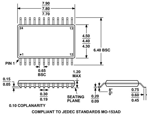
Figure 34. 24-Lead Thin Shrink Small Outline Package [TSSOP]
