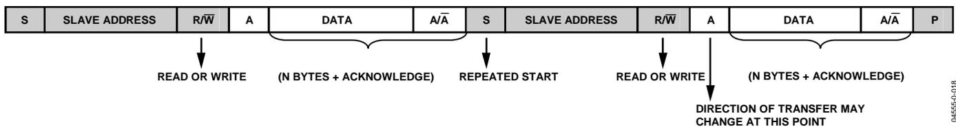
Figure 18. Combined Transmit/Read
