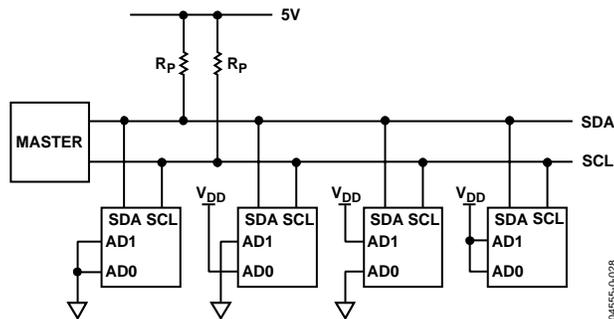
Figure 28. Multiple AD5255 Devices on a Single Bus
