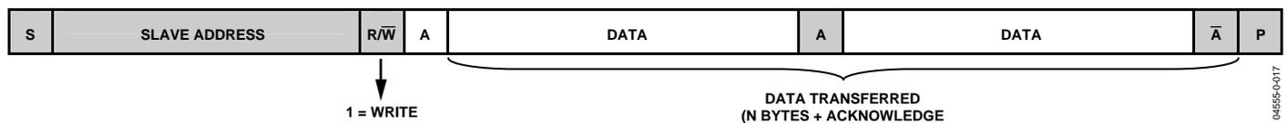
Figure 17. I<sup>2</sup>C—Master Reading Data from Slave
