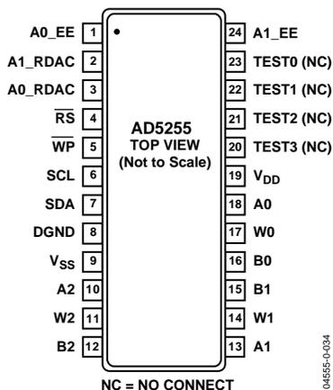
Figure 3. Pin Configuration
