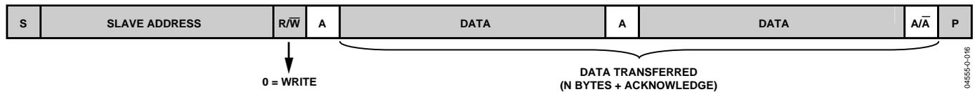
Figure 16. I<sup>2</sup>C—Master Transmitting Data to Slave
