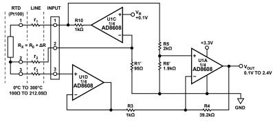
Figure 2. RTD Signal Conditioning Circuit Using a Three-Wire Connection
