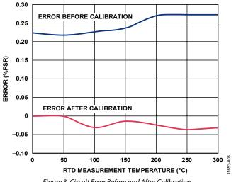
Figure 3. Circuit Error Before and After Calibration
