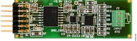
Figure 5. Photo of EVAL-CN0337-PMDZ Evaluation Board
