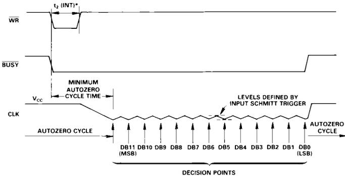
\* $t_2(INT)$  IS THE MINIMUM WRITE PULSE WIDTH WHEN USING INTERNAL CLOCK. SEE TIMING SPECIFICATIONS.
