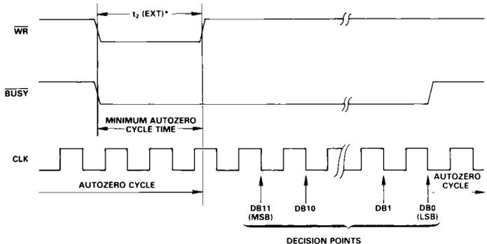
\* $t_2(EXT)$  IS THE MINIMUM WRITE PULSE WIDTH WHEN USING EXTERNAL CLOCK. SEE TIMING SPECIFICATIONS.
