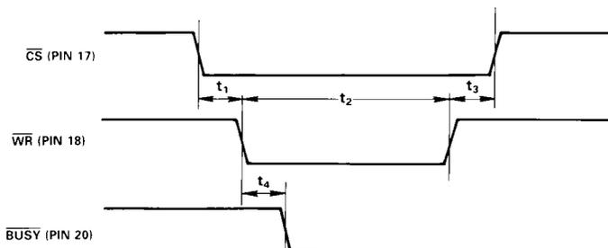
Figure 1. Start Cycle Timing
