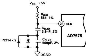
Figure 6. Circuitry Required for Internal Clock Operation
