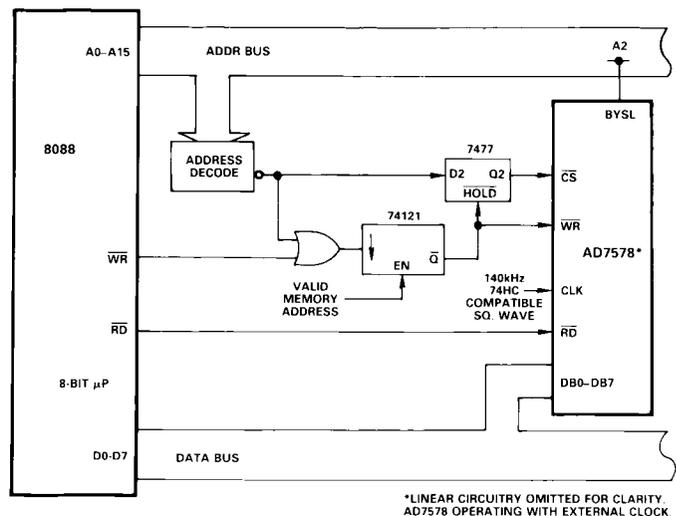
Figure 20. Interface to AD7578 Using External Clock
