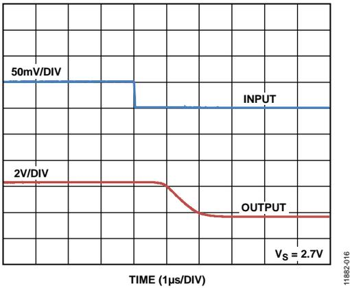
Figure 17. Differential Overload Recovery, Falling ( $V_S = 2.7\text{ V}$ )
