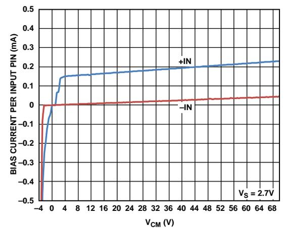
Figure 9. Bias Current per Input Pin vs.  $V_{CM}$
