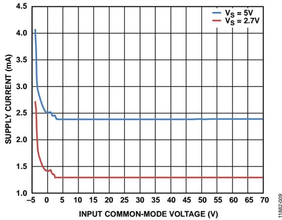
Figure 10. Supply Current vs. Input Common-Mode Voltage
