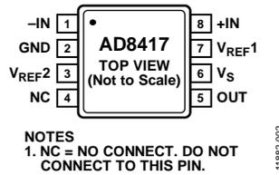
Figure 2. 8-Lead MSOP and 8-Lead SOIC\_N Pin Configuration
