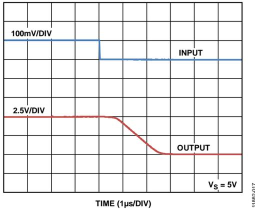
Figure 18. Differential Overload Recovery, Falling ( $V_S = 5\text{ V}$ )
