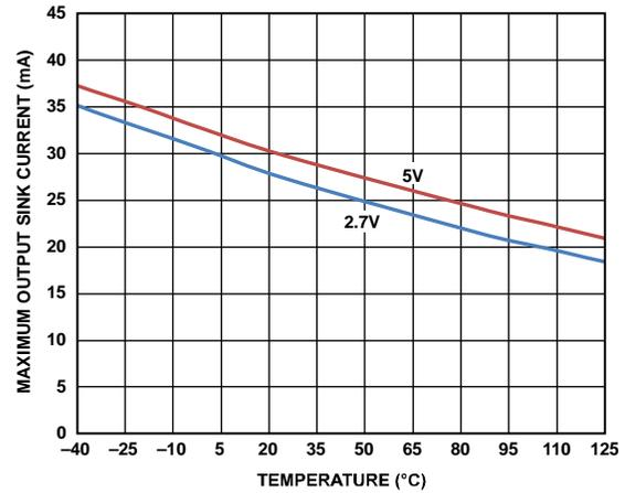
Figure 20. Maximum Output Sink Current vs. Temperature
