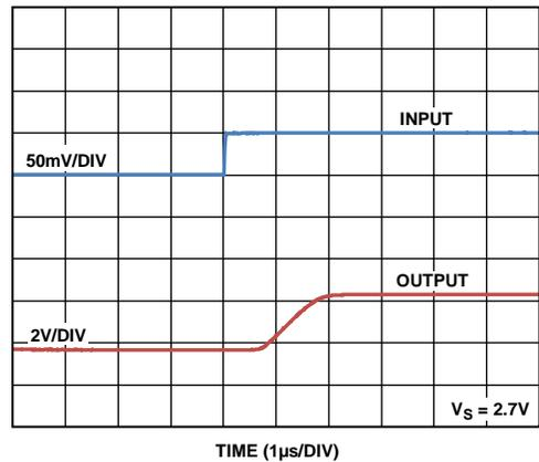
Figure 15. Differential Overload Recovery, Rising ( $V_S = 2.7V$ )
