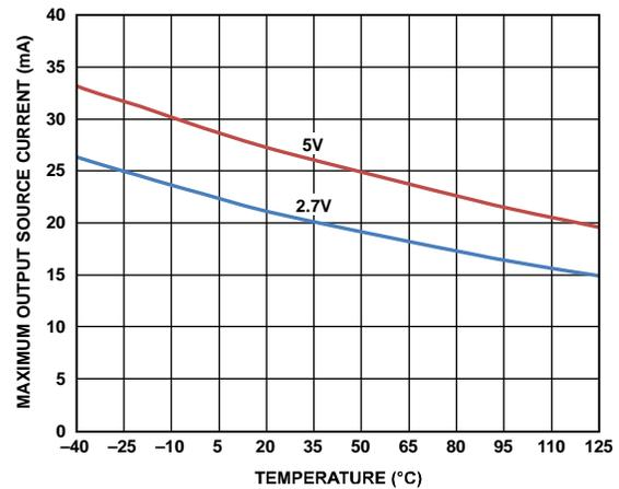
Figure 21. Maximum Output Source Current vs. Temperature
