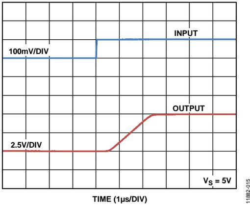
Figure 16. Differential Overload Recovery, Rising ( $V_S = 5\text{ V}$ )
