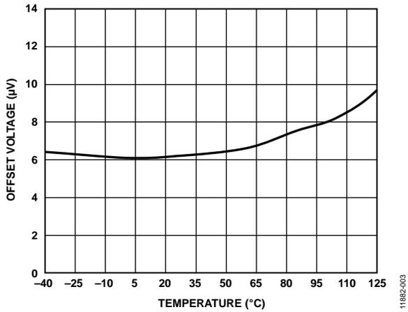
Figure 4. Typical Offset Voltage Drift vs. Temperature
