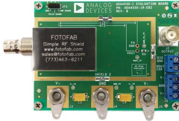
Figure 21. Evaluation Board Top View with SHIELD1
