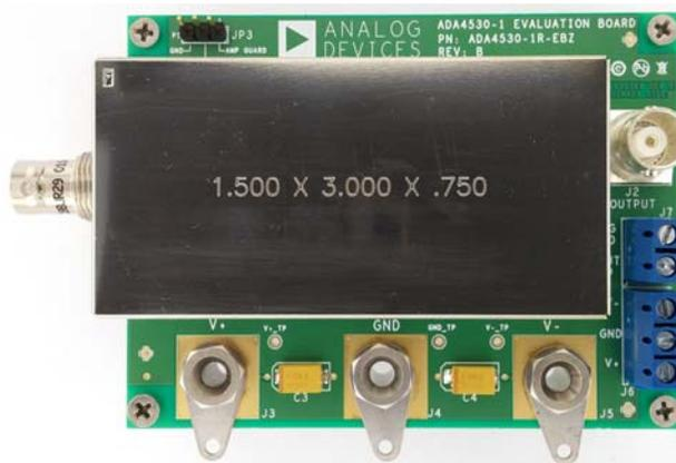
Figure 23. Evaluation Board Top View with SHIELD2
