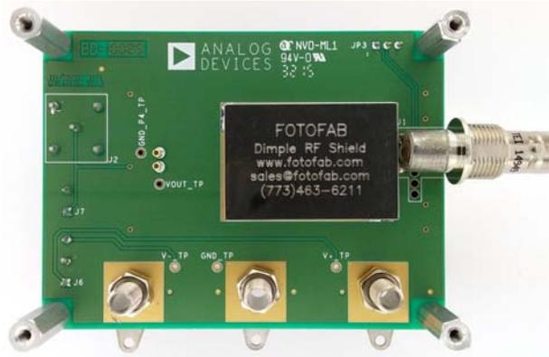
Figure 22. Evaluation Board Bottom View with SHIELD3
