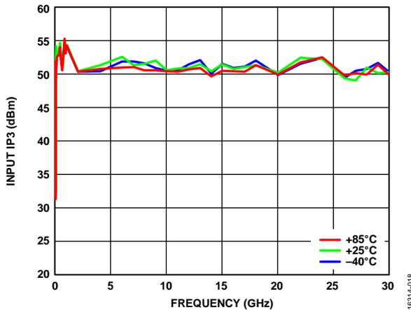
Figure 18. Input IP3 vs. Frequency over Various Temperatures
