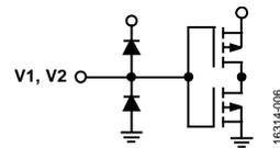
Figure 6. Digital Pins (V1 and V2) Interface Schematic
