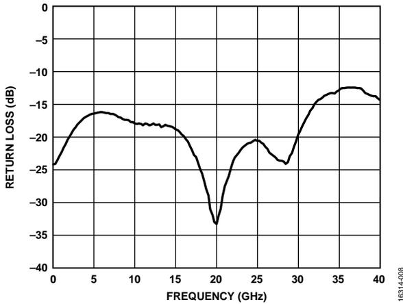
Figure 8. Return Loss vs. Frequency for RFC
