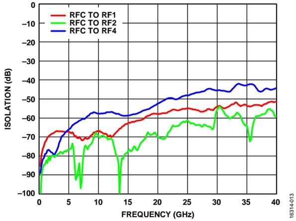
Figure 13. Isolation vs. Frequency, RFC to RF3 On
