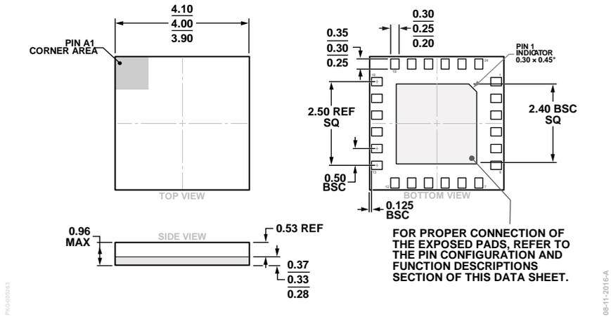
Figure 28. 24-Terminal Land Grid Array [LGA] (CC-24-4)
