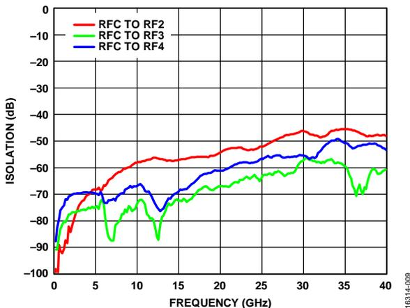
Figure 9. Isolation vs. Frequency, RFC to RF1 On
