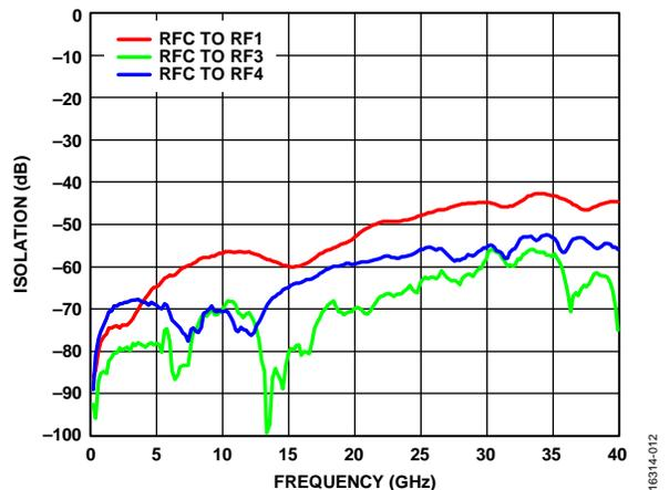
Figure 12. Isolation vs. Frequency, RFC to RF2 On
