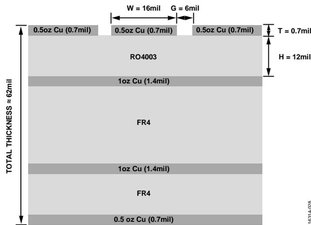
Figure 26. Probe Matrix Board (Cross Sectional View)
