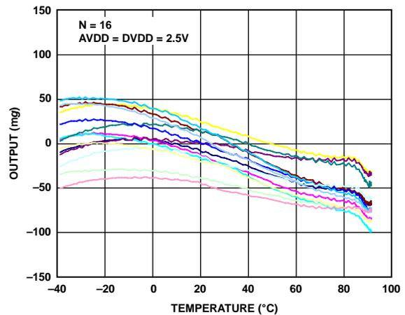
Figure 9. Z-Axis Zero g Offset vs. Temperature—
