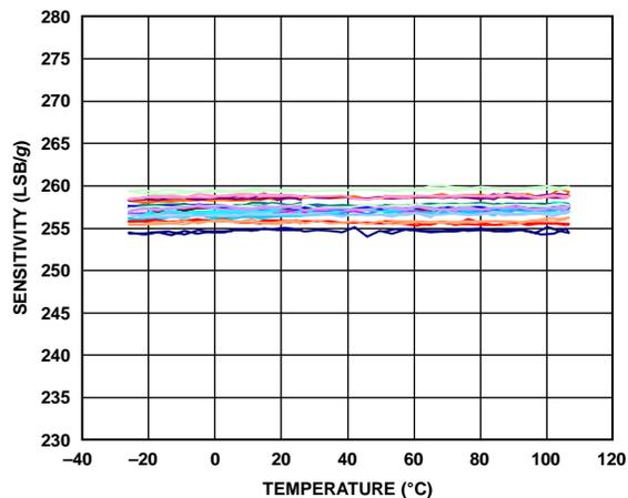
Figure 14. Y-Axis Sensitivity vs. Temperature—
