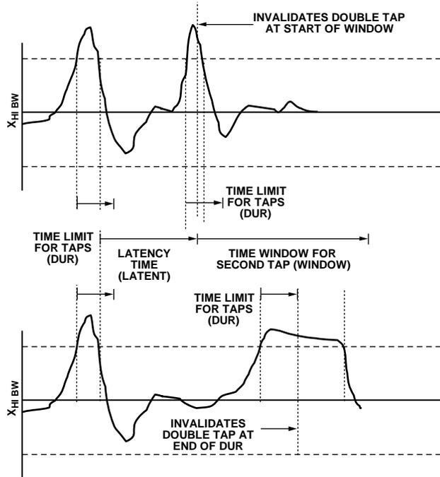
Figure 38. Tap Interrupt Function with Invalid Double Taps
