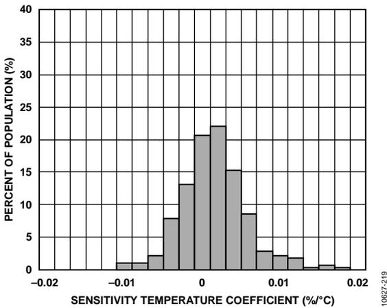
Figure 11. Sensitivity Temperature Coefficient,  $V_S = 2.5$  V, All Axes
