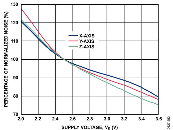
Figure 43. Normalized Noise vs. Supply Voltage,  $V_s$
