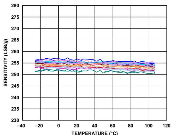
Figure 15. Z-Axis Sensitivity vs. Temperature—
