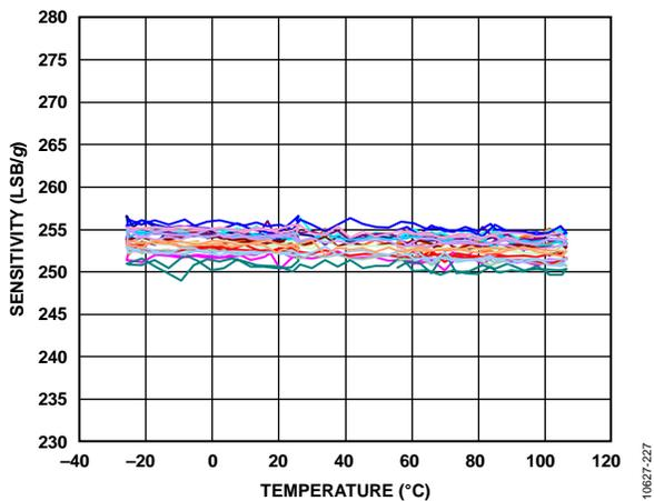
Figure 18. Z-Axis Sensitivity vs. Temperature—
