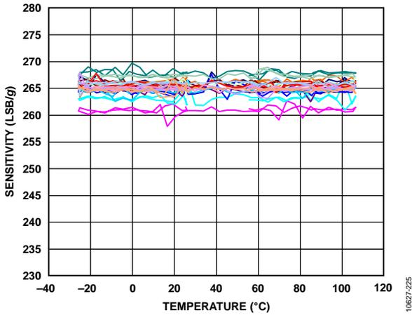
Figure 16. X-Axis Sensitivity vs. Temperature—
