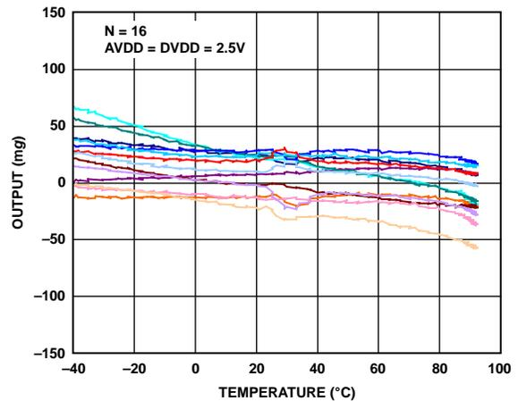
Figure 8. Y-Axis Zero g Offset vs. Temperature—
