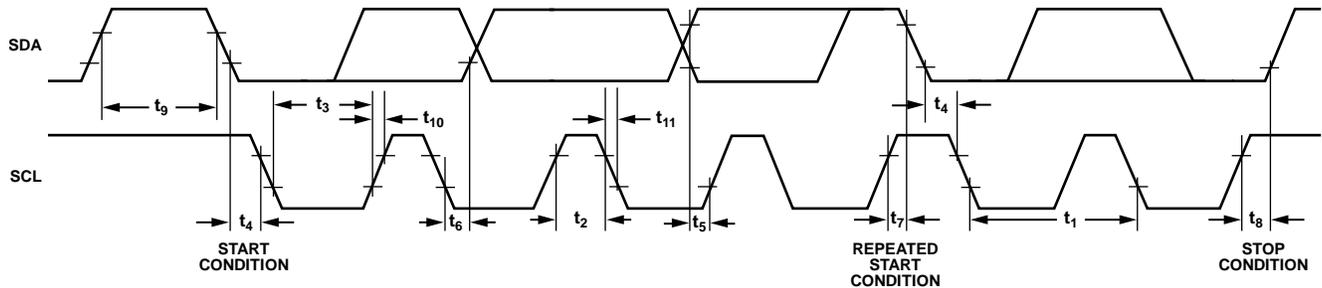
Figure 32. I<sup>2</sup>C Timing Diagram
