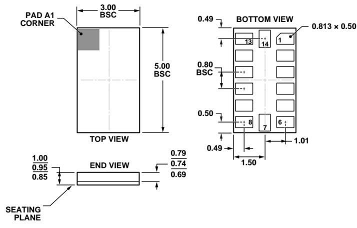
Figure 51. 14-Terminal Land Grid Array [LGA]
