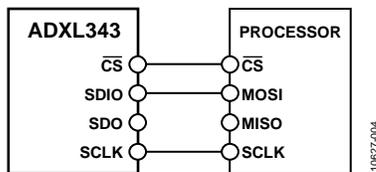
Figure 24. 3-Wire SPI Connection Diagram
