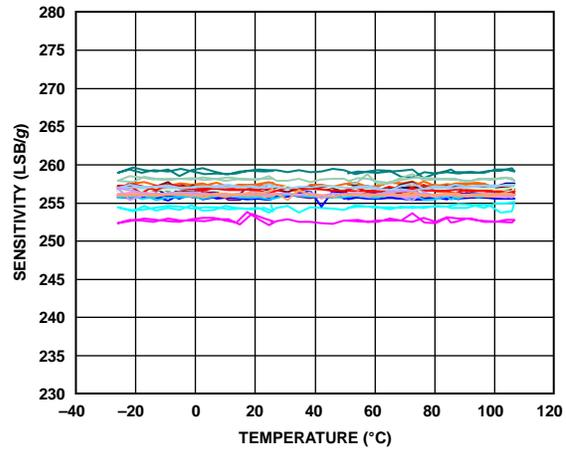
Figure 13. X-Axis Sensitivity vs. Temperature—
