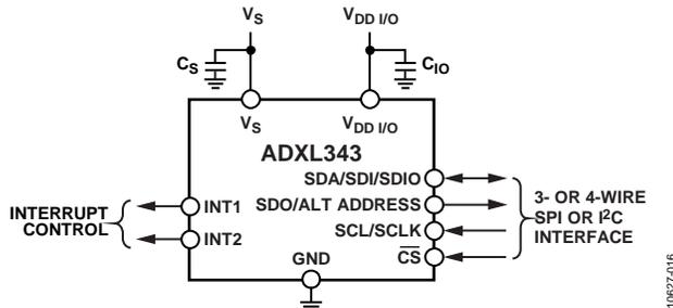
Figure 34. Application Diagram
