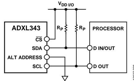
Figure 30. I<sup>2</sup>C Connection Diagram (Address 0x53)
