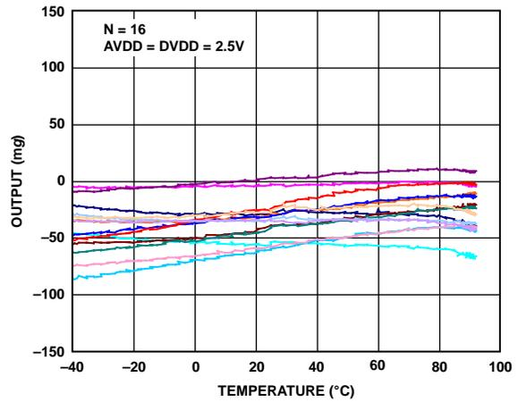
Figure 7. X-Axis Zero g Offset vs. Temperature—
