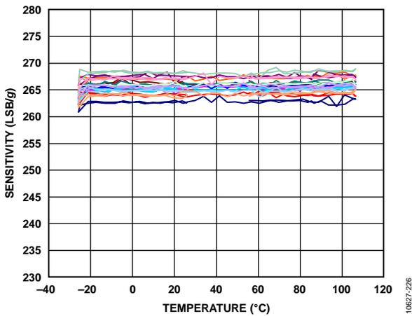
Figure 17. Y-Axis Sensitivity vs. Temperature—
