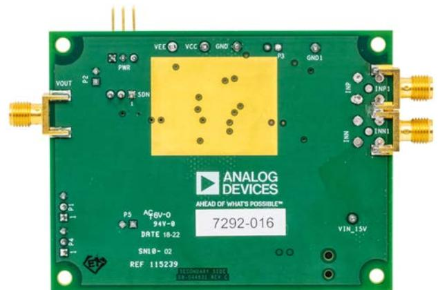
Figure 2. Evaluation Board, Bottom
