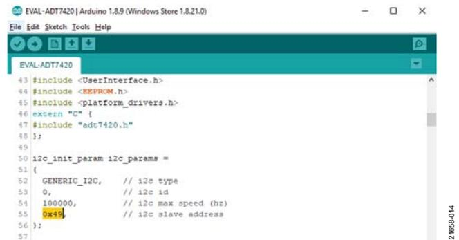
Figure 15. Arduino IDE Code Change
