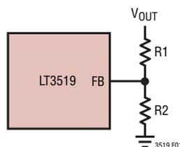
Figure 1. FB Resistor Divider for Boost LED Driver
