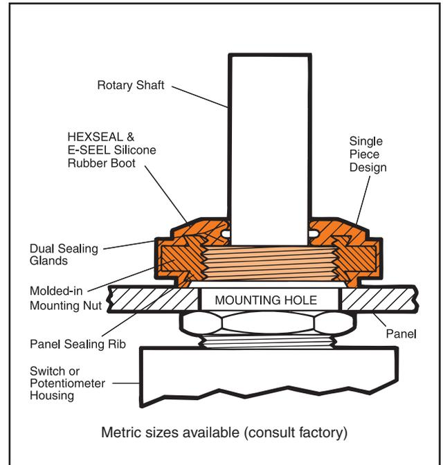
FIGURE 21 Rotary Shaft Seals – IP66/68 Rated
