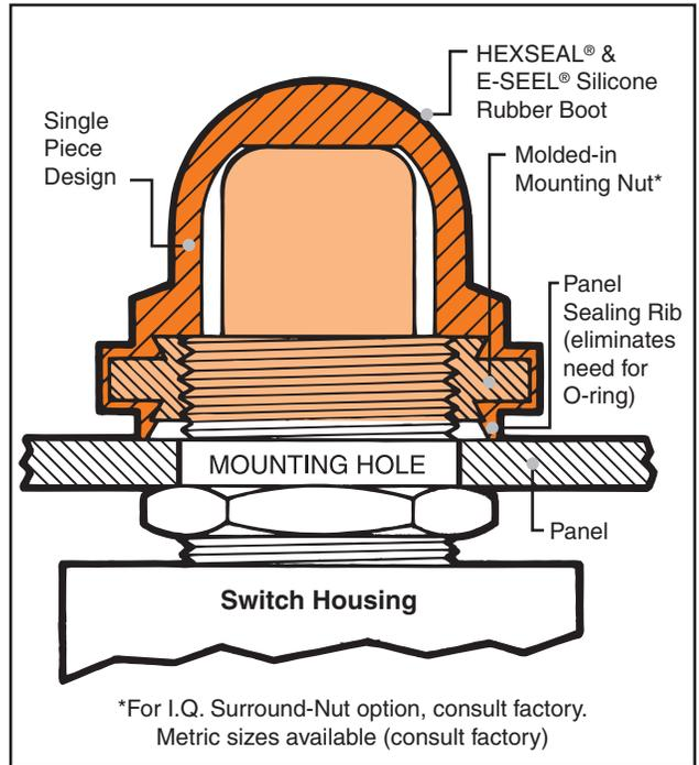
\*APM's policy is to manufacture our HEXSEAL® sealing boots as defined by the requirements of MIL-Spec B-5423 which we regard as the standard for the switch, circuit breaker and potentiometer industry. These requirements were formulated based on our original patent.
