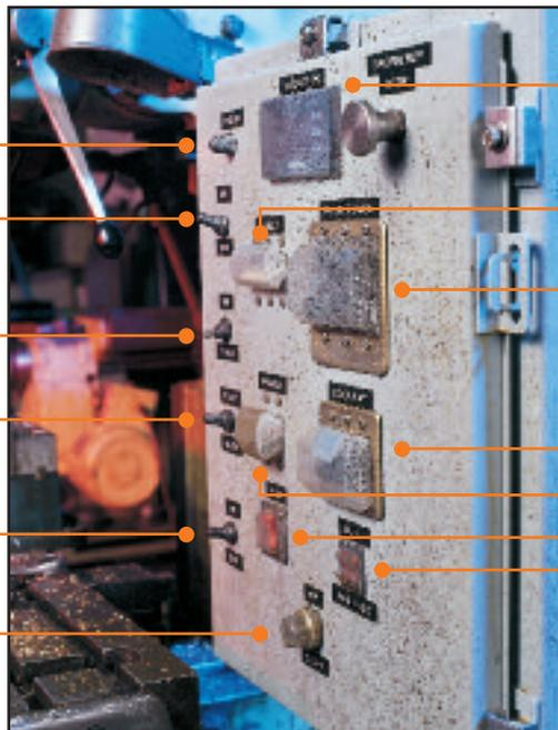
Lever style back-of-panel mounted circuit breaker boots
