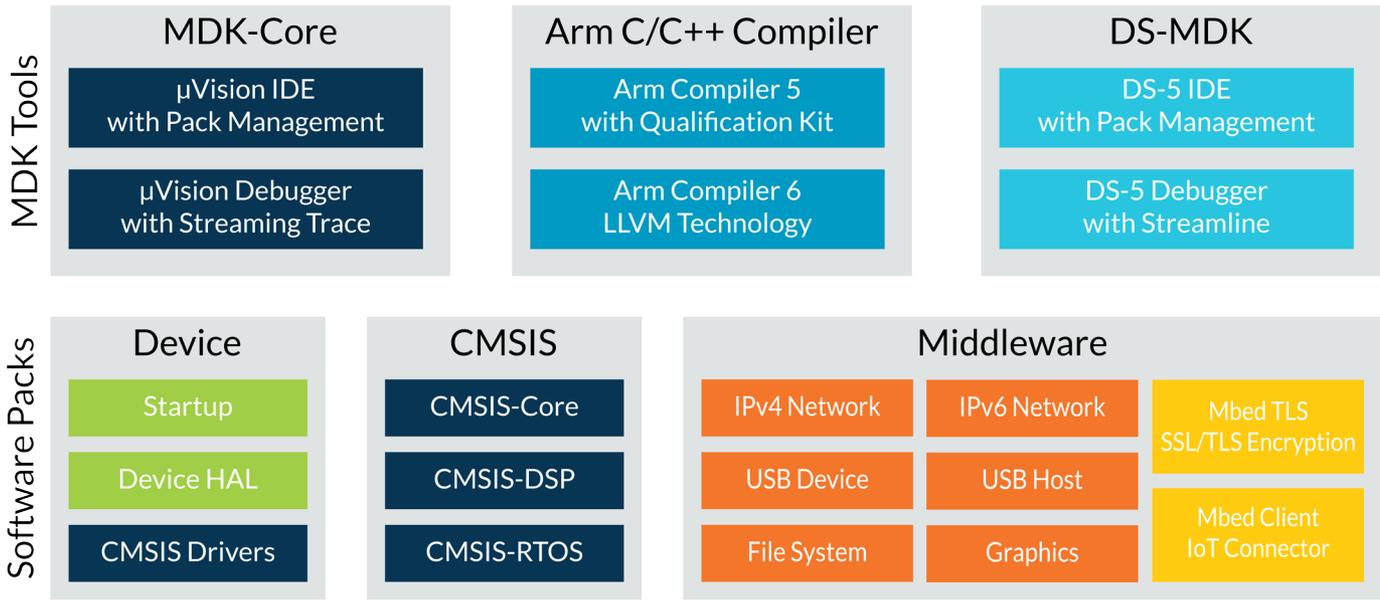
MDK-Core offers leading support for over 3,750 Cortex-M based devices including the new Arm Cortex-M23/M33 cores. The μVision debugger includes event recorder and component viewer to show run-time behavior of software components. Together with the ULINKpro™ debug adapter, it offers full instruction trace and complete code coverage information.
