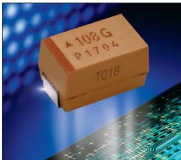
Low ESR, high capacitance and high ripple current are the key parameters for processor filtering. Multianode configuration within a standard E case package meets these requirements. Parameters such as ESR 15mΩ, capacitance 1500μF and ripple current above 4A rms makes TPM series ready to use with the latest processor families.
