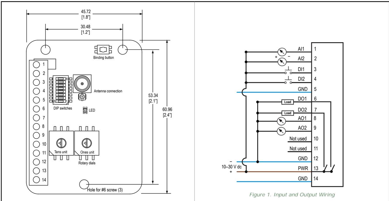
Figure 1. Input and Output Wiring
