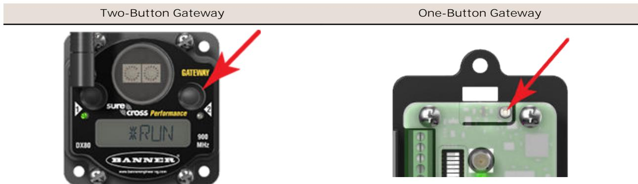
The LEDs flash alternately when the Gateway is in binding mode. Any Node entering binding mode will bind to this Gateway.
