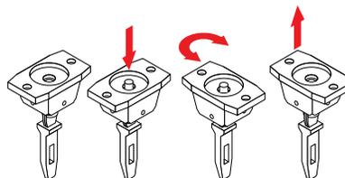
The flexible actuator mounting flange may be rotated 90° with respect to the actuator position. To rotate, push the flange in the direction of actuation, turn the flange either direction, and release to lock the flange in the new position; see the diagram above.
