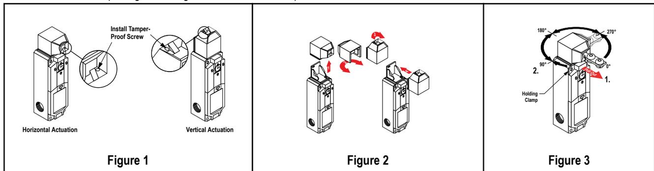
**Rotating Actuator Head to Desired Position**
