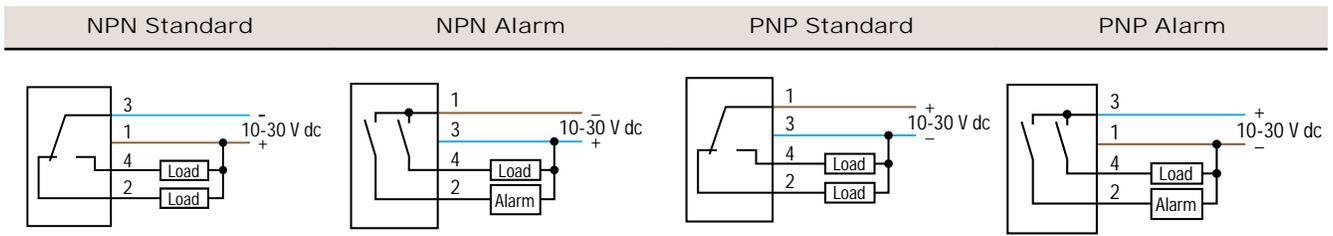
Wiring for the quick disconnect (QD) models is functionally identical.
