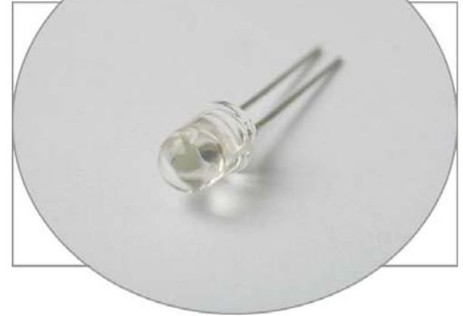
Bivar's 5mm T1 3/4 Package 5UWC Series LED may be used in almost any application. They are offered in 6500K color temperature and come in multiple intensity, viewing angle, and body styles. Bivar offers a water clear LED lens for maximum light output. The Flange LED is ideal for Panel Mount Clip & Ring assemblies and the Standard LED is ideal for vertical spacer and holder assemblies.
