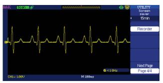
Monitor and analyze long-term signal behavior by recording data continuously over an extensive period of time and playing it back for post acquisition analysis. Data is recorded in a sequence of up to 2500 frames.
