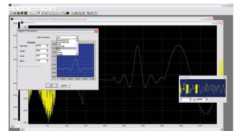
Use waveform editing software to easily generate, edit, and download custom arbitrary waveforms. Generate waveforms by importing a text file, or define via freehand, point draw, or waveform math. Waveforms can also be loaded from the generator for documentation purposes.
