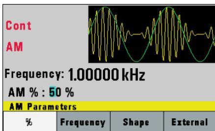
The 4045B provides AM and FM modulation along with linear/logarithmic sweep and built-in counter capabilities. Internal and external sources can be used for triggering and modulating the signal.
