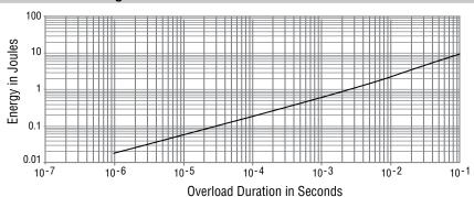
The energy absorbed by the resistor expressed in Joules can be calculated by multiplying the peak power of the pulse in watts times the length of the pulse in seconds.
