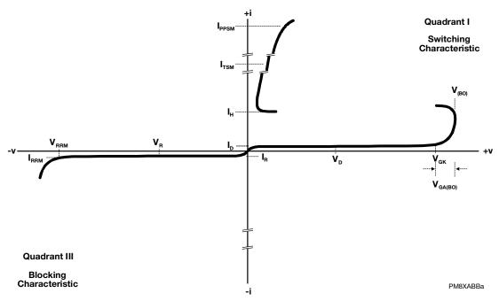
Figure 2. TISP8201HDM AK Terminal Characteristic
