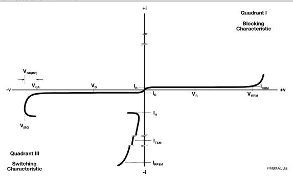
Figure 1. TISP8200HDM KA Terminal Characteristic
