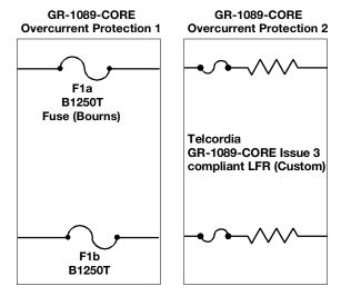
Figure 4. Typical Overcurrent Protection
