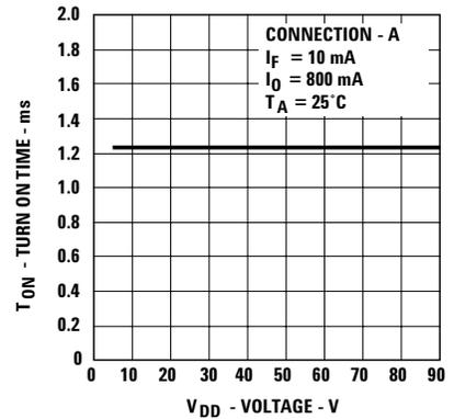
Figure 13. Typical Turn On Time vs. Voltage.
