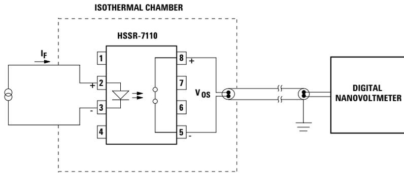
Figure 19. Voltage Offset Test Setup.
