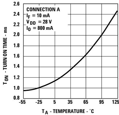
Figure 11. Typical Turn On Time vs. Temperature.
