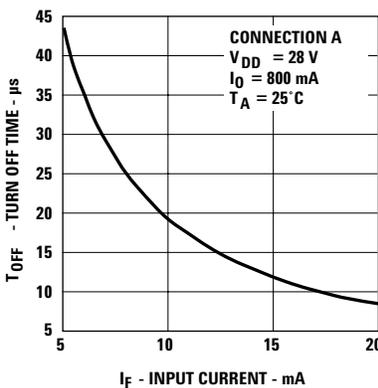
Figure 15. Typical Turn Off Time vs. Input Current.
