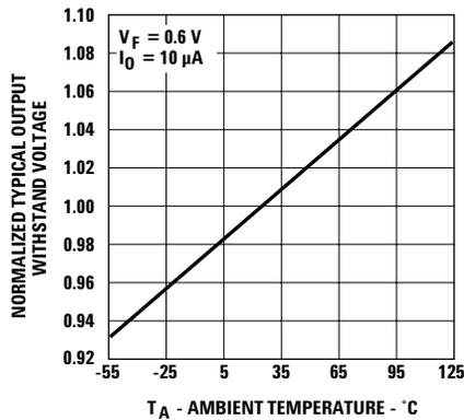
Figure 5. Normalized Typical Output Withstand Voltage vs. Temperature.
