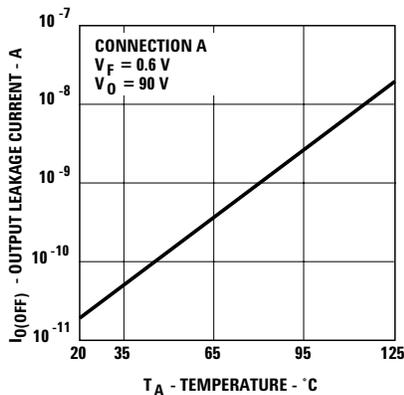
Figure 8. Typical Output Leakage Current vs. Temperature.
