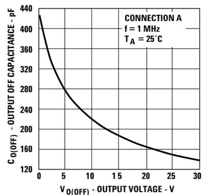
Figure 16. Typical Output Off Capacitance vs. Output Voltage.
