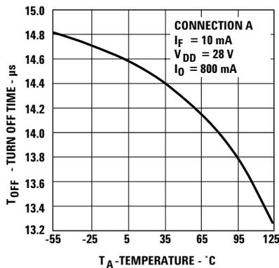
Figure 14. Typical Turn Off Time vs. Temperature.
