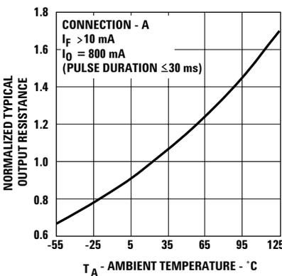
Figure 6. Normalized Typical Output Resistance vs. Temperature.
